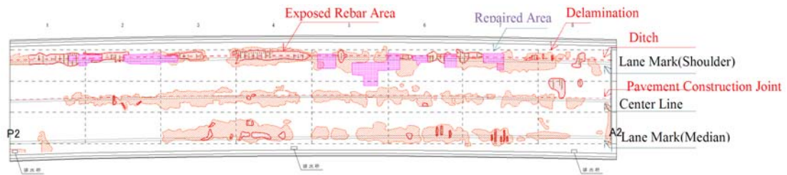
Figure 6. Slab Surface of Bridge E (Upper slab surface after pavement removed)
