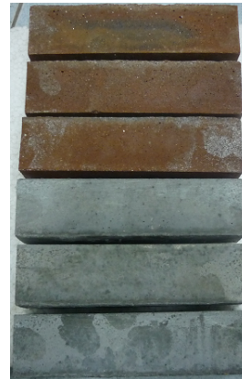
Figure 3. GPM samples before and after firing at 1000 °C
