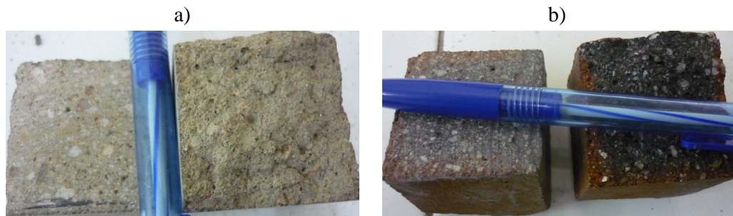
Figure 4. Colour change in the cross section of samples fired at 1000 °C a) PCM samples, b) GPM samples
