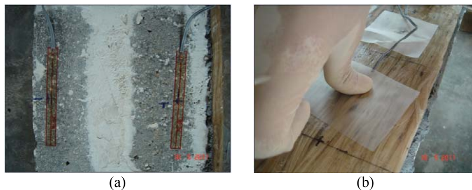
Figure 3. Location of strain gauge- (a) Side surface of the beam. (b) Polymer strain gauge on strengthening composites laminate.
