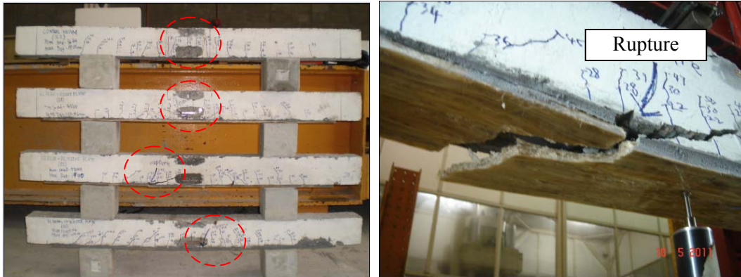
Figure 9. Structural failure mode
