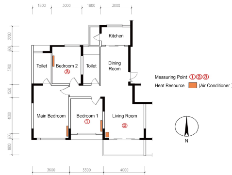
Figure 1. Measurement spots in the plan of test house A
