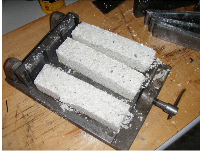
Figure 1. Photos of insulating samples based on PUR waste and waste of EPS granulate
