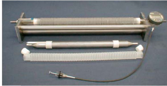
Figure 2. Dilatometer bench with accessories used to determine autogenous shrinkage
