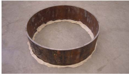
Photo 12: Ring used for the in-place percolation test
