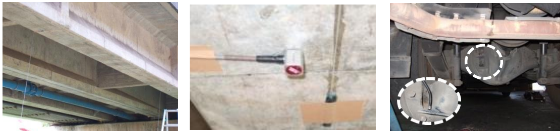
Figure 5. Details of main girders (bottom view) and sensor location on a girder and the bus
