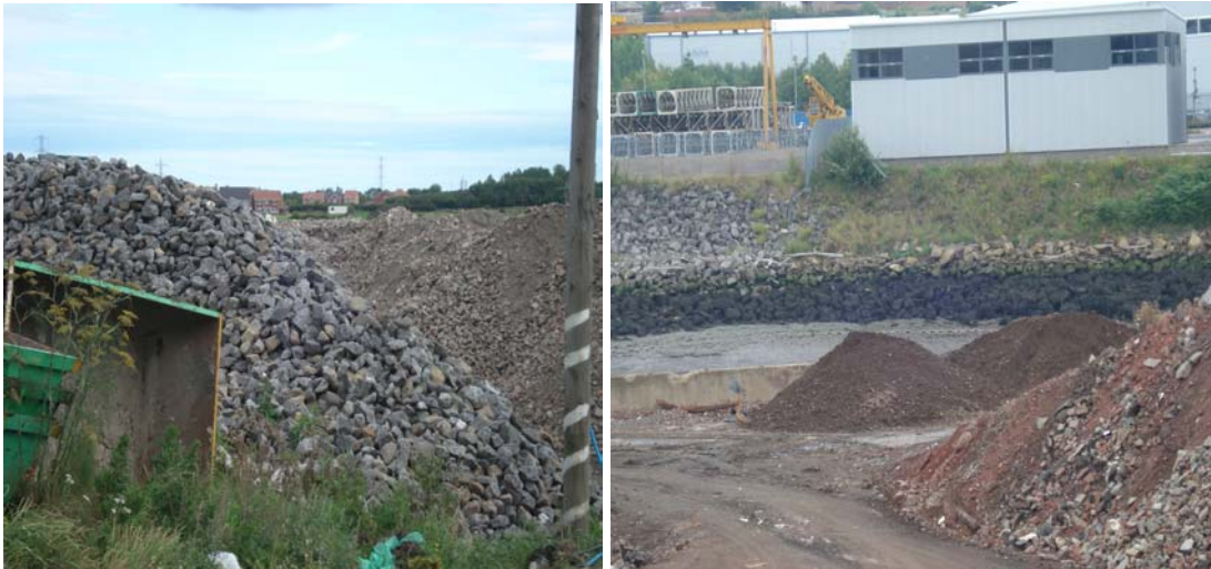
Figure 2. Concretes crushed in to different size of aggregates.
