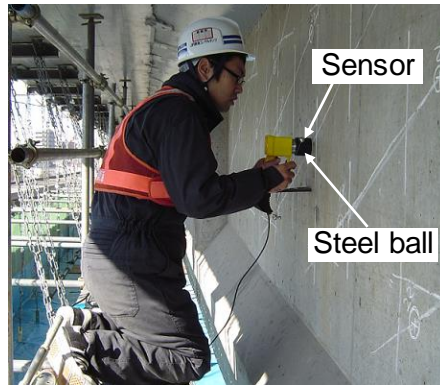
Figure 16. Outline of measurement using the method focused on frequency characteristics
