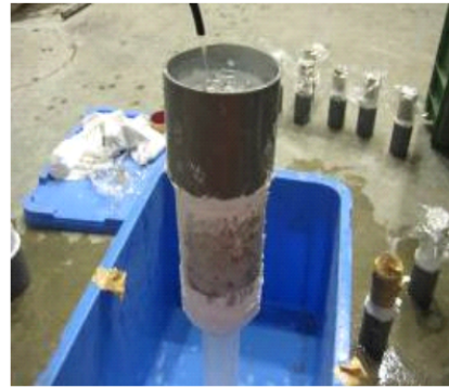
(b) Measurement of water leakage
