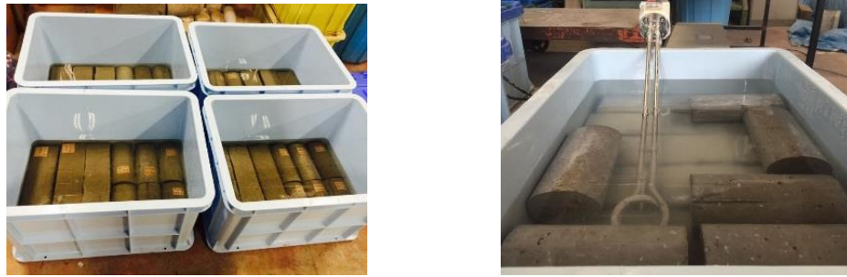
Figure 2. Alkali exposure followed by immersion in NaCl solution
