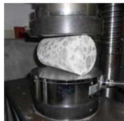
Figure 5. Splitting Tensile Test
