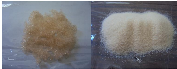
(1) Original granules of IERs (2) Grinded and sieved powders of IERs
