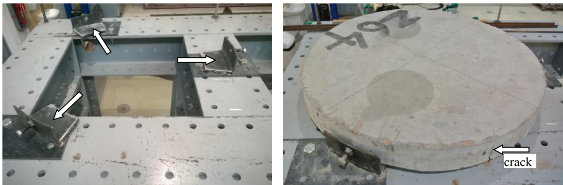
Figure 2. Three supports of the tailored lab stand for impact tests and a slab during the test
