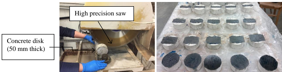
Figure 1. Slicing concrete cylinder
