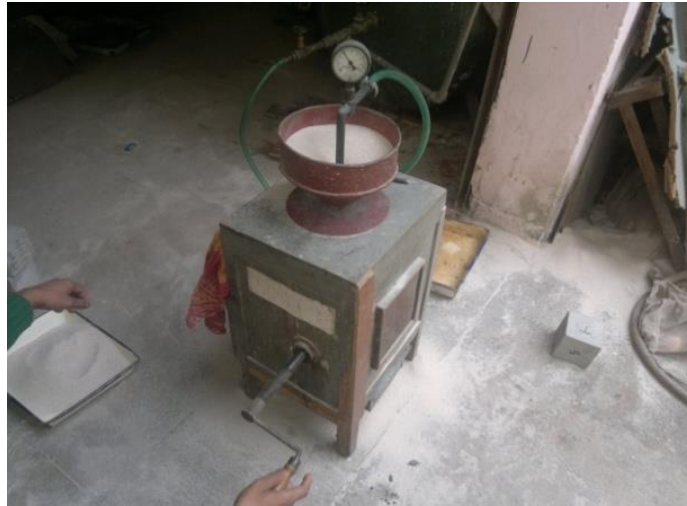
Figure 3. A Concrete Specimen under Abrasion Testing
