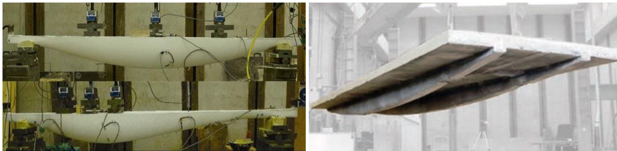
a. Optimised beams [Bailiss 2006]
