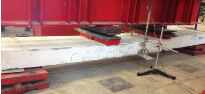
Figure 5. Typical One Way Slab under Testing.
