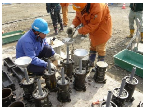
(a) Pre-placed aggregate concrete
