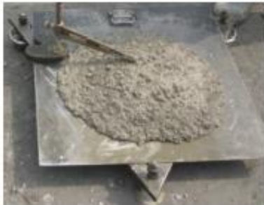
Figure 14. Situation of the Slump Flow Test Construction.
