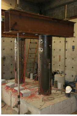
Figure 6. Large-Scale CFTs Sustained Loading Experimental Test Setup
