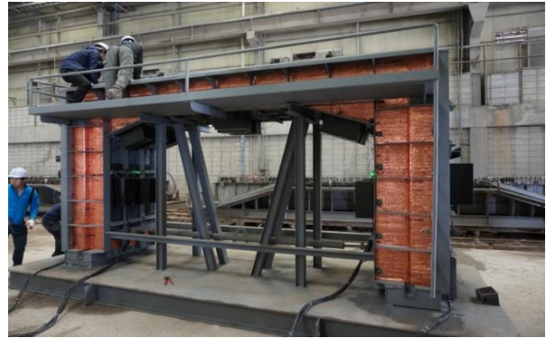
(b) Steel Form for Microwave Heat Curing
