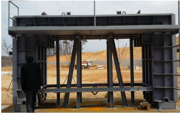
Figure 3. (a) Steel Form for Steam Curing
