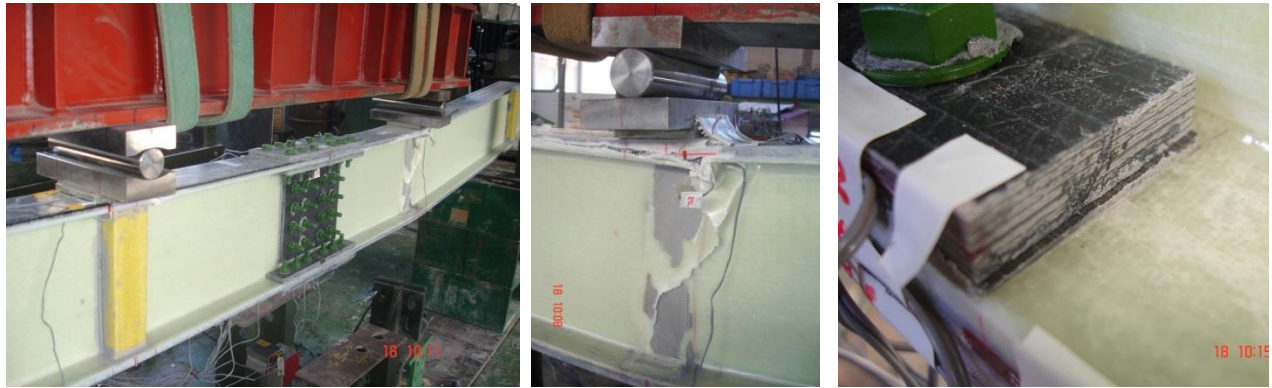
Figure 6. Failure modes of specimen FH-1
