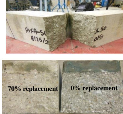
Figure 9. Fracture Surface Appearance.
