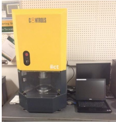
Figure 6. Gyrotory Intensive Compaction Tester (ICT).
