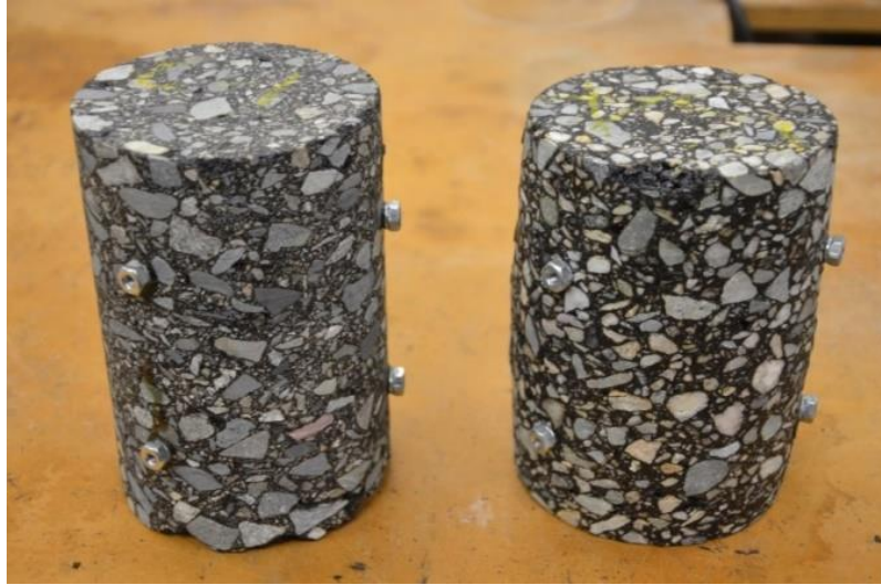
Figure 3. Flow Number Sample before (left) and after (right) Testing
