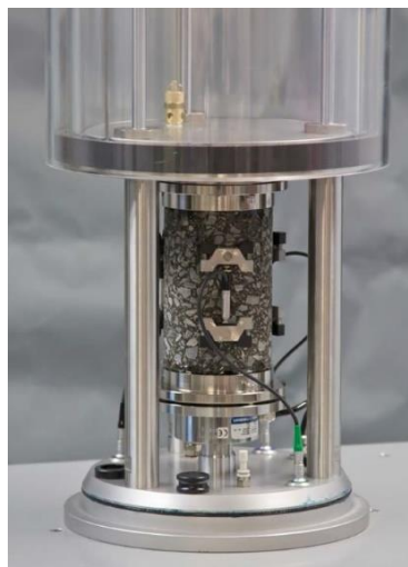
Figure 2. Dynamic Modulus Tested by Asphalt Mixture Performance Tester (AMPT)
