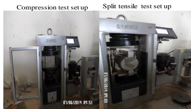
Figure 1. Testing set up for compression and tensile strength
