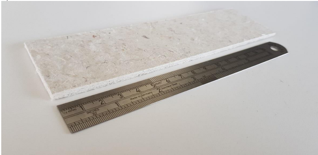
Fig. 7. a) Air-laid non-woven feather fibre samples. b) Feather fibre board manufactured by hot-pressing the air laid non-woven sample in a) at 6 MPa and 154 °C for 60 seconds.
