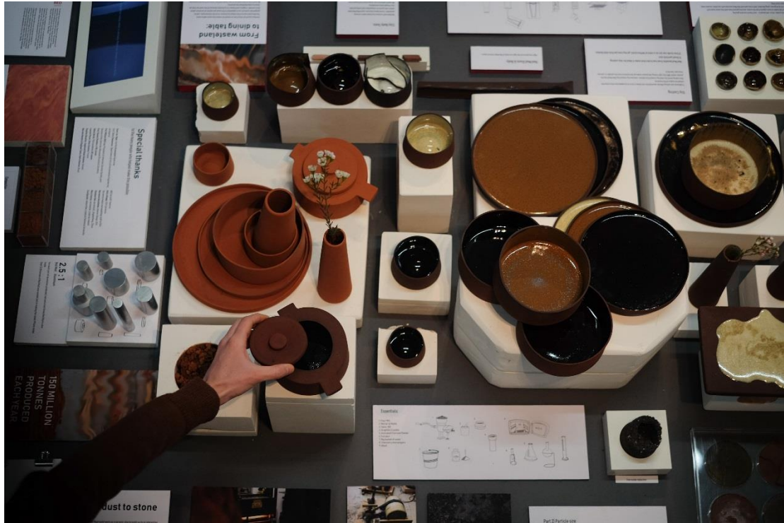
Fig. 2. A selection of ceramic products manufactured by Royal College of Arts students using red mud.
