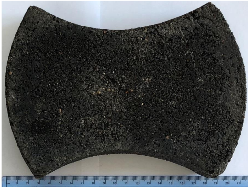
Fig. 6. Sand plastic block made from waste LDPE in the Cameroon.
