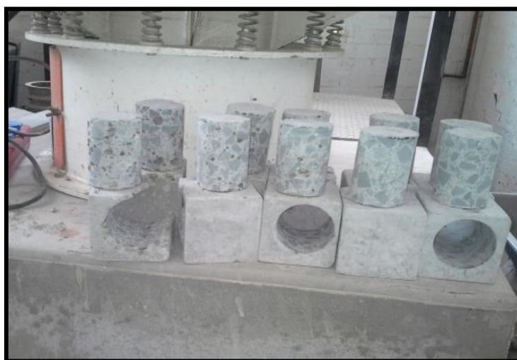
Figure 1: Cored concrete samples
