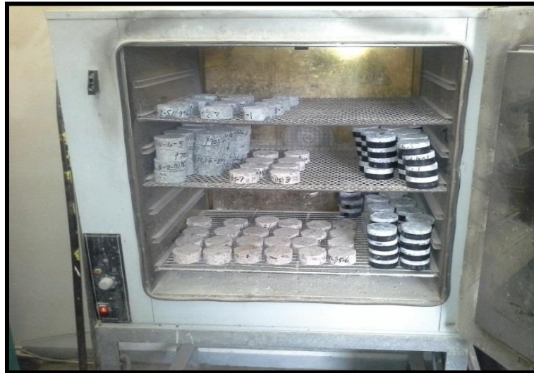
Figure 2: Prisms samples for durability index tests
