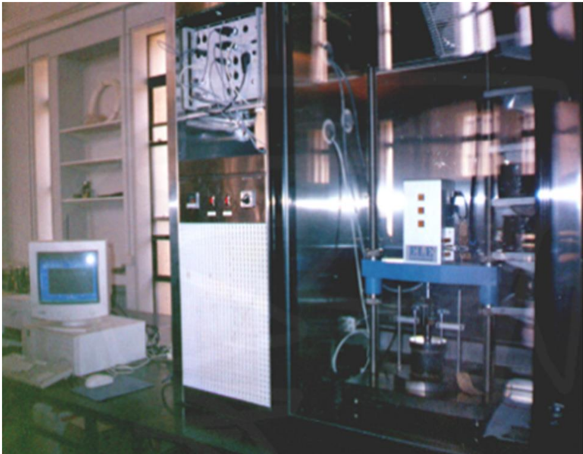
Figure1. Universal Testing Machine (UTM) and Environmental Chamber
