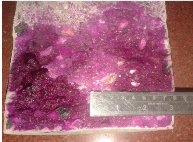
Fig.2: Measurement of carbonation depth
