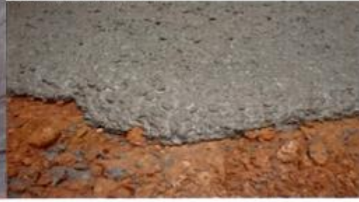
Fig. 2: The SCC mixture exhibited no segregation or bleeding even after a high-energy drop chute placement in the 70 m (230 ft) deep shaft
