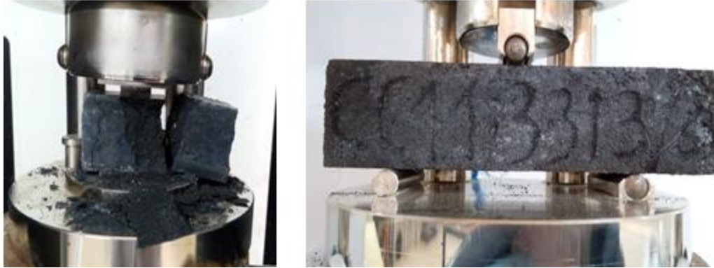
Fig. 1. Compressive Strength Test of Half Prism And Flexural Strength Test of Prism.
