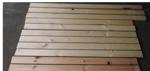
b) Cut and planned lamellas
