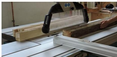
a) Processing of salvaged timber
