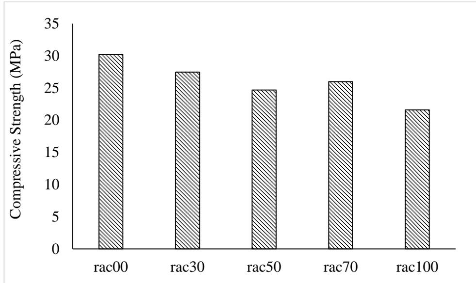
Figure 5: Variation in concrete compressive Strength for the specimens under uniaxial compression.
