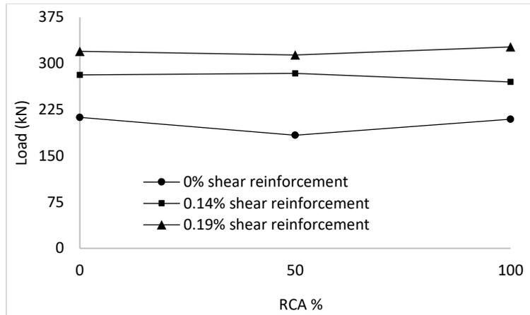
Figure 2: Shear Strength variation with replacement ratio and shear reinforcement (*S.Ignjatović, B.Marinković and Tošić 2017*)
