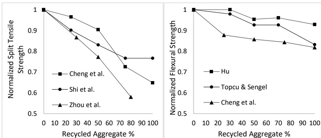
Figure 1: Split Tensile Strength (Cheng GY 2005) (Shi W and Hou JP 2001) (Zhou JH, et al. 2010) & Flexural Tensile Strength (Hu 2007) (Topcu IB and Sengel S 2004) (Cheng GY 2005)
