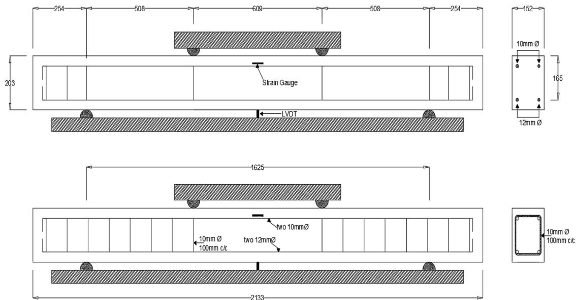
Figure 4: Reinforcement Detail for Beam Specimens.
