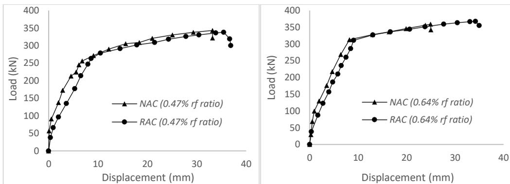
Figure 3: Response of beam specimens having reinforcement ratios (*Arezoumandi, et al. 2015*)
