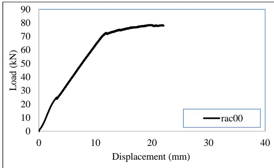
Figure 8: Response of Flexure Critical RAC00 specimen
