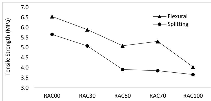
Figure 6: Variation in concrete tensile splitting strength for the specimens.
