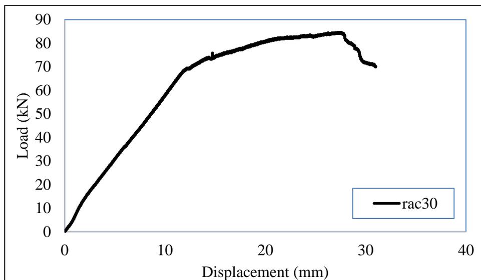
Figure 10: Response of Flexure Critical RAC30 specimen.
