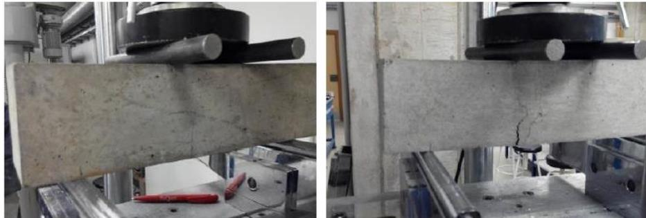
Figure 3. Specimen with first crack (left) and final breakage (right)
