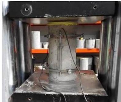
Figure 1. Specimen in the toughness compression test
