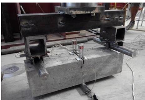
Figure 5. Arrangement of specimen after cracking in flexural tensile strength test
