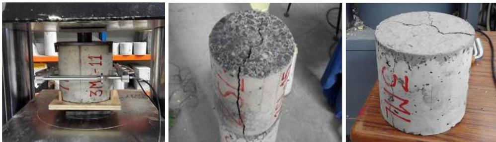
The results of cracking load by unit of area,  $f_{ct}$ , showed that Figure 4. Barcelona test set-up (left) and radial cracks in specimens after the test (center and right)
