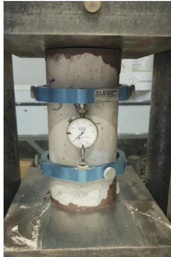
Figure 4. MOE test setup
