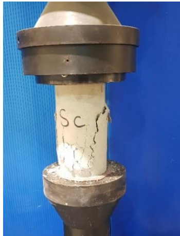
Figure 1. Compressive strength test setup
