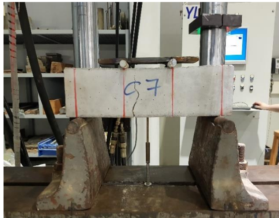
Figure 3. Flexural capacity test Setup
