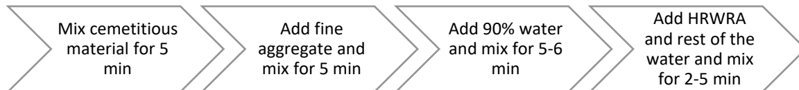
Figure 2: Mixing procedure of UHPCs
