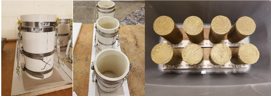
(a) (b) (c) Figure 4 (a) Specimen mold; (b) Three molds tied to a plywood board; and (c) Specimens in a box under curing
