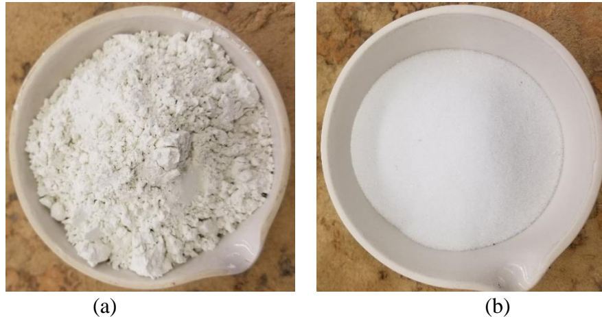
Figure 3. (a) ACAS glass powder; and (b) CS-30 glass sand
