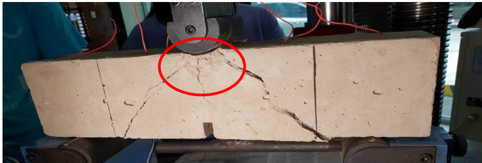
Figure 6. Strain localization of AAC beams
