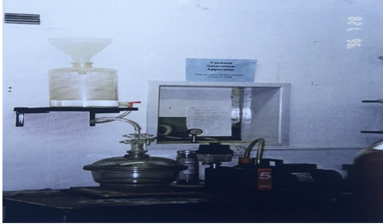
Figure 4: Vacuum Saturation Apparatus
