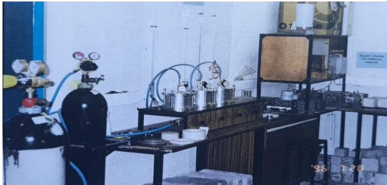
Figure 3: Gas Permeability Apparatus
