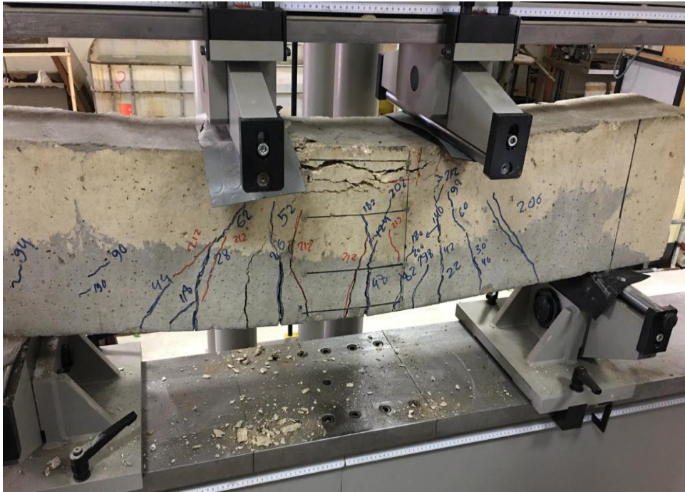
Figure 14. Damage pattern for beam (B1)
