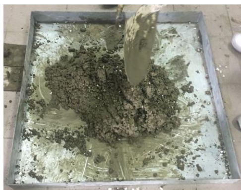
Figure 7. Mixing of concrete
