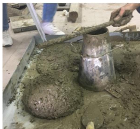
Figure 8. Control mix slump
