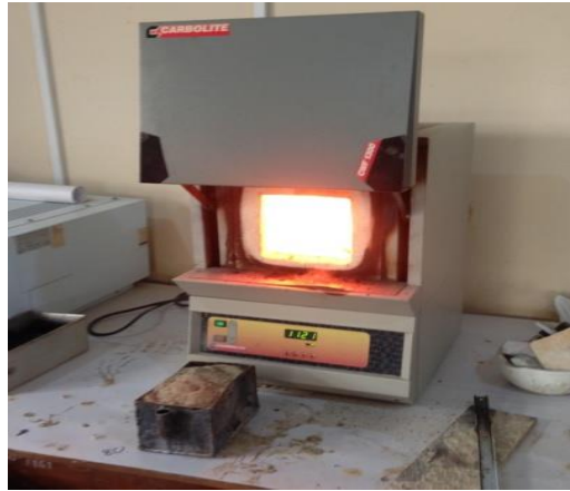
Figure 3: Incineration of materials inside the furnace
