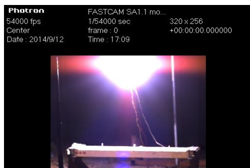
(a) Blast test on OPSC panel
