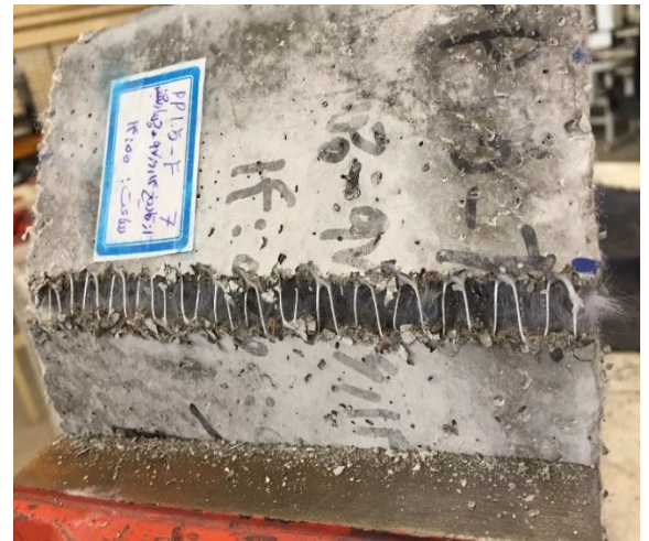
Fig. 4 How fibreglass net placed in
