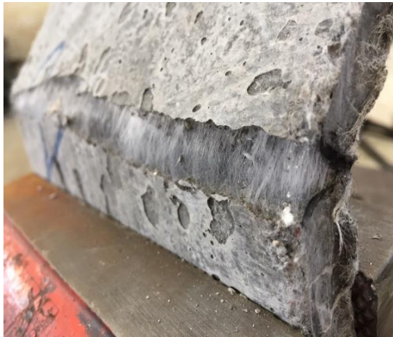
Fig. 3 Distribution of polypropylene fibres specimens
