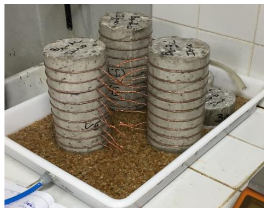
Fig. 3. Experimental device for the capillary imbibition test
