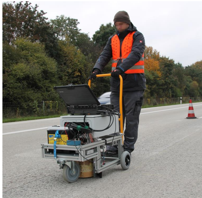
Fig. 3. Prototype of the impact-echo scanner used on a concrete pavement slab.
