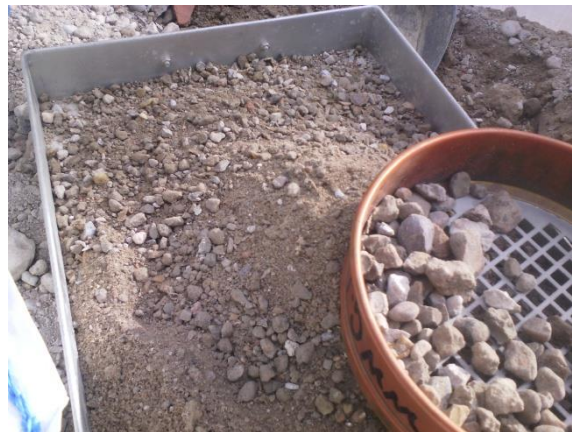
Figure 2: Sieving crushed concrete particles into 20mm maximum size
