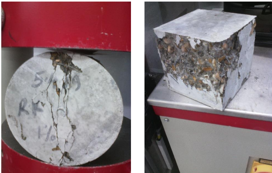
Figure 8: Failure mode of steel fibre reinforced concrete in tensile and compression
