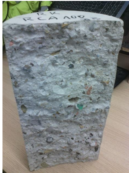
Figure 7: Failure surface of RCA100
