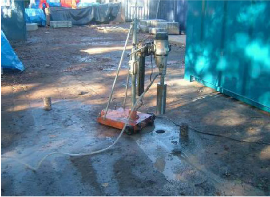
Figure 128. Core sample taken from middle and end part of the trial car park at the Lowdham Grange site .
