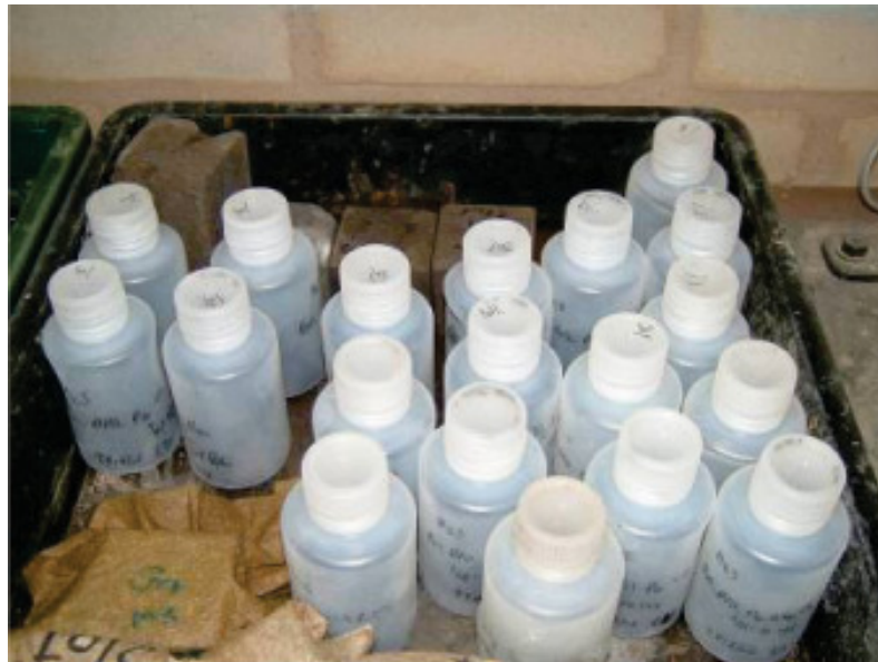
Figure 62. Plastic bottles containing paste specimens for H 2 S check.
