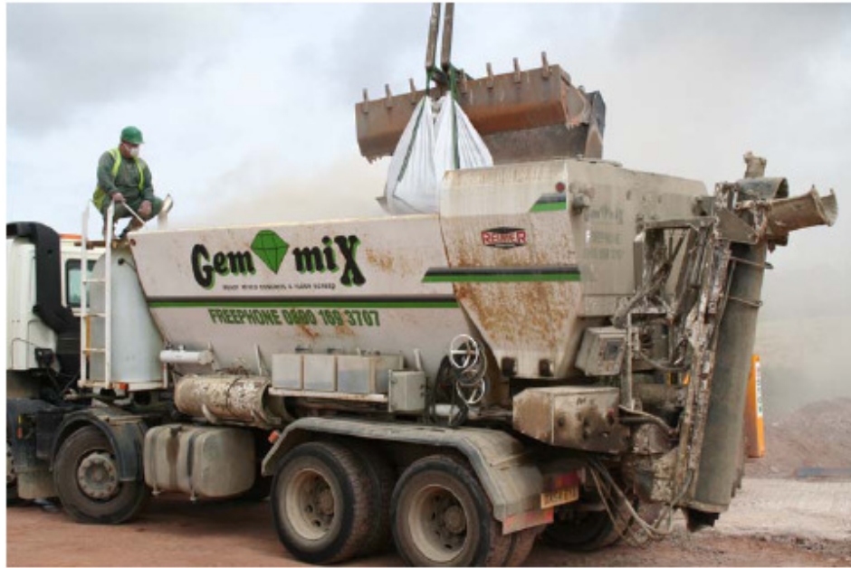
Figure 115. Loading the mixer with blended powder.
