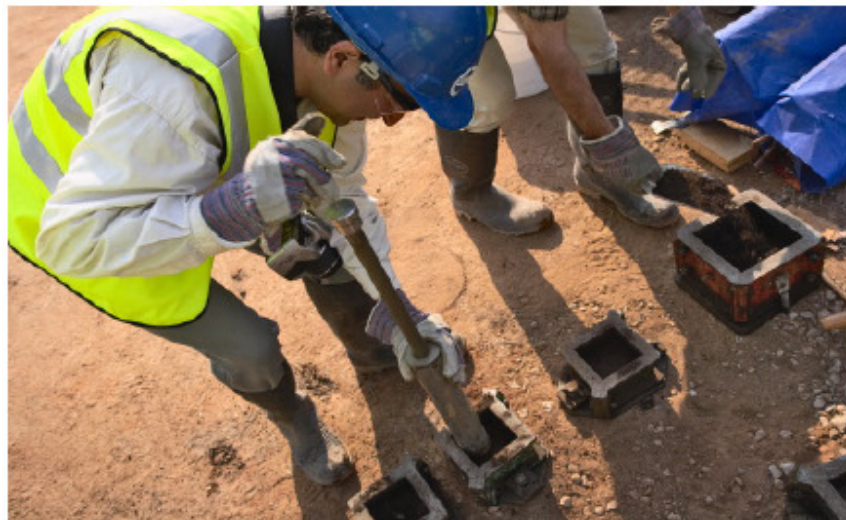
Figure 113. Sampling the stabilised soil.
