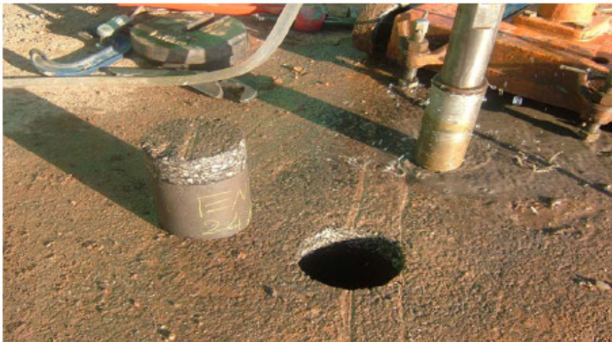
Figure 124. Core sample taken from the lower part of trial road at the King's Mill Hospital site.
