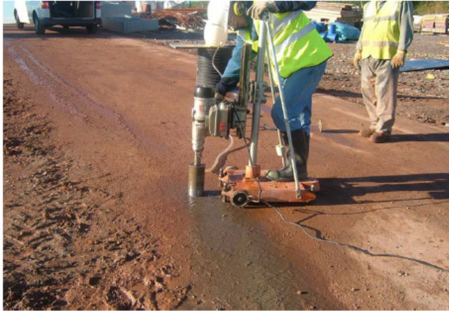
Figure 123. Coring machine used to drill the cores at the King's Mill Hospital site.
