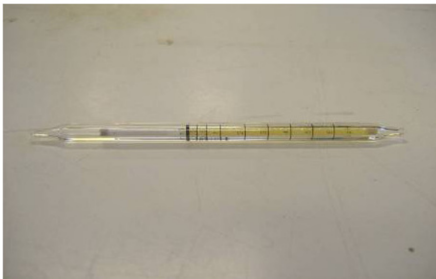
Figure 68. Drager Accuro H 2 S detection tube.
