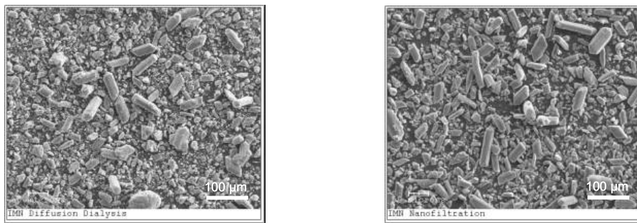
Figure 2. Microphotographs of gypsum from DD (left) and NF (right) purified acids
