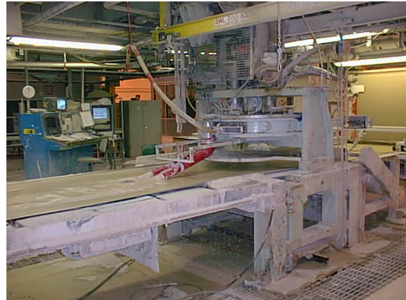
Figure 5. (Top photo) gypsum slurry is applied to the bottom sheet of paper and then the top sheet of paper is applied (bottom photo).
